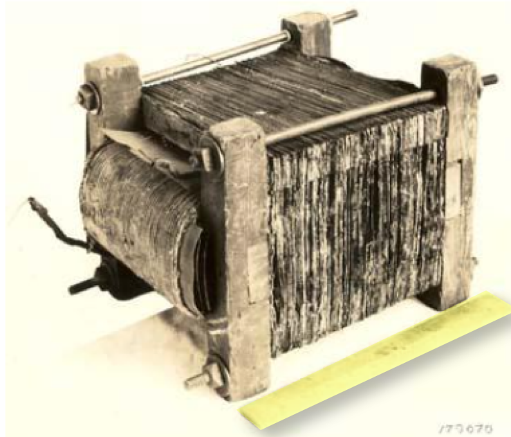
FIGURE 8. The Stanley transformer used in Great Barrington, 1886. The transformer’s copper windings are wrapped around a paper mold whose curved ends protrude a bit beyond the wooden frame’s four end pieces. The wooden frame is bolted together top-and-bottom, on both sides. The middle arms of the E-shaped iron plates extend through the windings, alternating from one side to the other, opposite side. The top and bottom arms of the E plates may be discerned as dense narrow shapes outlined at the top and the bottom of the figure. The ruler placed in right foreground indicates the unit is about one foot long. [SOURCE: https://edisontechcenter.org/GreatBarrington.html ]
