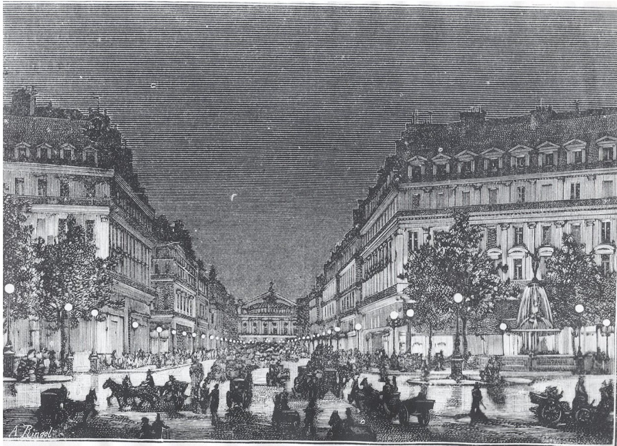
Figure 2: The Avenue de l'Opéra lit up by Yablochkov “candles” or arc lamps in 1878 during the Exposition Universelle, France’s third “World’s Fair.” SOURCE: https://commons.wikimedia.org/wiki/File:L%27avenue_de_l%27op%C3%A9ra_eclair%C3%A9e_par_les_lampes_Jablochkoff.jpg
