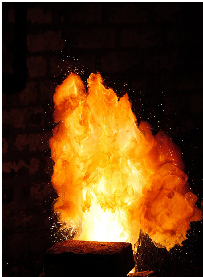
Figure 20. A controlled thermite reaction of aluminum and manganese oxide.
