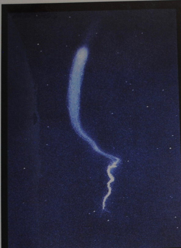
A chemical trail like the one here – this one deployed from a sounding rocket at night as opposed to in the daytime – will help researchers track wind movement to determine how it affects the movement of charged particles in the atmosphere. Credit: NASA
